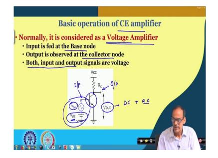
So, yeah so, what we have the CE amplifier again we will be just touching the basic operation, but before that I must say that, whenever we call the common emitter amplifier. the input it is fed at the base of the BJT and then output it is observed at the collector node. So, you can see that the input we are feeding here and then output we are observing at the collector node.
