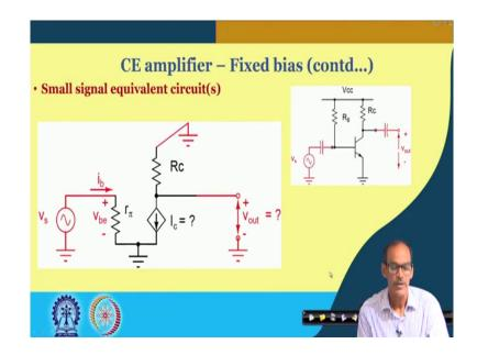
So, in the next slide we can look into the corresponding small signal side equivalent circuit. But let me take a break and then we will be discussing in detail on this one.
