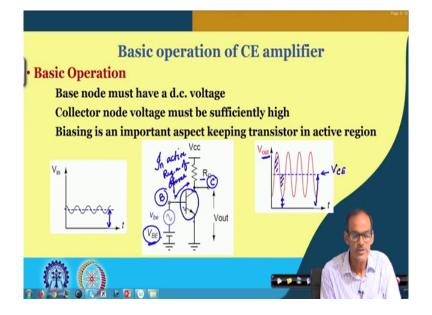
So, what we are considering now practical circuit biasing circuit. So, what we have it is the requirement wise as I said that the input, we do have signal which is riding over a DC voltage. In this case we are calling this is V be. So, likewise at the output we do have a DC voltage, so we need to remove those things.
