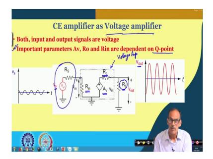
So, let us go little detail of that so, in the next slide we will be discussing that, but here as I say that since you are looking for the circuit as a as a voltage amplifier. Typically, this is a small signal model of the voltage amplifier right.
