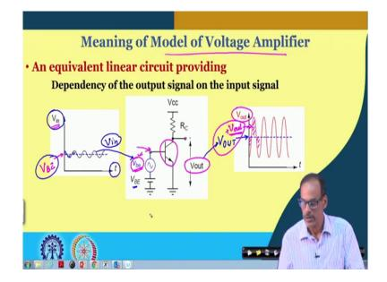
What we have here as I said that, we do have the basic amplifier and at the input we are having a DC voltage, on top of that we do have we are applying a small signal. So, if you observe the voltage here and if we call this is V in to the circuit; it is having a DC part here which is capital V B E and then on top of that we do have the small signal part. So, you may say that the small signal part is given here, and that small signal part is the small V b e or you may call this is small v in.
