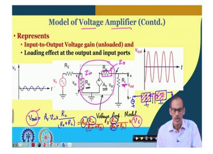
So, this is what the same thing we have discussed, we do have the model, we do have the model of the amplifier; namely the voltage model, voltage amplifier rather, voltage amplifier model. So, what it represents is basically the input to output relationship. And as I said again to summarize the, it is having three important parameters called input resistance, voltage gain and the output resistance.
