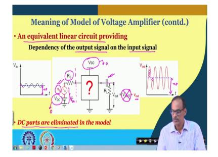
So, what we mean by the voltage amplifier? It is an equivalent linear circuit and it is main purpose is to provide the dependency of output signal on the input signal. So, dependency of this output signal on the whatever the input signal we are applying that supposed to be captured by this one.
