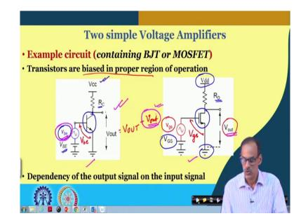
Say for example, the first one it is; it consist of BJT, second one it is having a MOS transistor. And for each of the cases what we have here it is, the DC voltage source and then of course the ground and along with the biasing element registered. The transistor it is in this case the BJT is kept in the active region of operation with the help of V B E, the DC voltage here.
