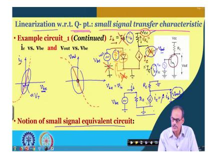
So, that is what we are saying that whenever we are talking about linearization basically it is with respect to operating point or Q point and which is referred as small signal transfer characteristic. So, in the small signal transfer characteristic; in fact, we do have two parts, we already have discussed, but one is a small signal i c with respect to small signal vbe voltage. In fact, this is exponential part exponential behavior.
