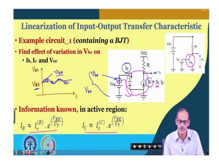
Now, let me go a little more detail of the linearization. So, what we are doing is basically we are making use of these two equations and then we are considering instead of considering this transistor we are considering the small signal equivalent circuit. And, then using this equivalent circuit we are considering this loop and then we are considering beta and then we are finding the corresponding output voltage.
