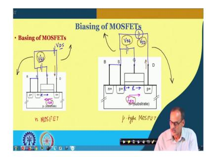
So, let us about think about the biasing. So, primarily we will be covering the n-MOSFET p-MOSFET, but just for our reference we are also keeping the n MOS structure. So, for your reference if you see this is n MOS and if you recall how we have biased it so, for proper operation gate is at higher potential by V GS and most of the time we prefer to keep this body and source connected together and then at the drain we do have another potential source we call V DS.
