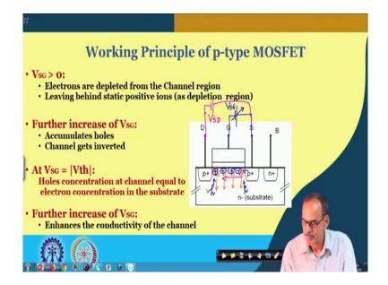
So, what is the working principle of the circuit and then that will be helping us to really derive the expression of the current in terms of explain the terminal voltages. So, quickly let us apply the voltages here. So, what we said is that this is the channel it is we have to make it p-type. So, it should be at gate should be at a lower potential than the source by V SG and we have to apply the V SD, yeah. So, we do have the V SD here which makes the drain side at lower potential.
