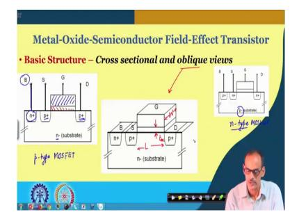
So, here the MOSFET for p-MOS type I should say where the channel it is and the channel it is supposed to be p-type and this is the cross sectional view of p-type MOSFET. Just for your reference I am also keeping the n channel MOSFET. So, I should say just for our reference we are keeping n-type MOSFET.
