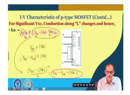
So, for significant V SD what you are expecting there it is the expression of the current it will be mu p into epsilon ox divided by t ox into W by L into V SG minus threshold voltage minus V SD similar to n-MOS device multiplied by V SD. Only difference is that instead of V SG there it was V GS and instead of V SD it was V DS, rest of the things it is similar; of course, we do have the mu also it is different, but we can think of it is just a constant.
