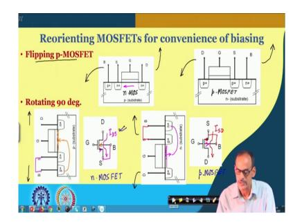
So, what kind of reorientation shall we do? First thing is that we will flip the p-MOS transistor, because here we do have lower potential and here we do have higher potential. And, so, source side as I said we can make it towards the ground and drain side we can make it out.
