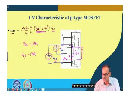
So, quickly let me apply the voltage. So, we have as I said for our convenience we have rotated the device. So, let me apply this V SG. Now, it is very convenient that the positive side of the potential source, we are connecting towards the upper side and this is V SG body is connected together; body is connected to the source and then we do have the V SD and the current it is flowing in this direction.
