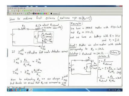
So, how to achieve fast criteria that means, extreme right correspond to R X equal to 0. So, how to achieve that? And so, how we will do it? So, this will be done by; so, let me draw this the draw the circuit. So, I am drawing these terminals because R X is an external element that will connect to the circuit and everything else is internal to the circuit internal to the ohmmeter ok.
