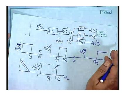
You are having, an up sampler and a down sampler, let me draw the diagram, there is a down sampler a value 3, and there is an up sampler 3. And then we are having three filters H 0, whose frequency domain characteristics, I will show, you H 0, H 1 and H 2 corresponding outputs are y 0 n, y 1 n and y 2 n, x n is the input. Now, the three, the three filter characteristics are given, H 0 is H 0 e to the power j omega.
