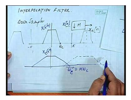
Similarly, the other one, that is when we are down sampling, we are flattening the base, suppose this is the original frequency spectrum all right, this again omega c. Now, if you are down sampling by a factor M, then the response of this, down sampled signal or compress signal will be, this is the first one is X e to the power j omega. So, X
