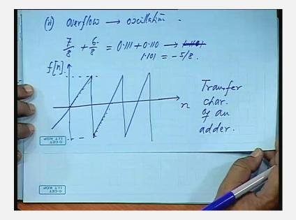
So, rounding of the product of multiplication that causes oscillation, now there are other types of oscillations due to overflow, this is because of the rounding off there can be also
