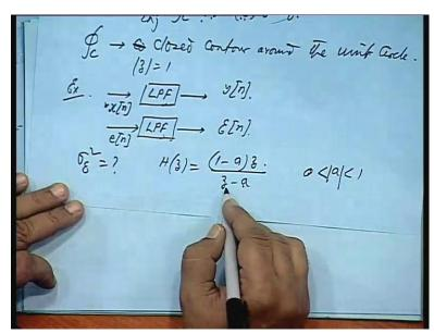
For sigma Epsilon squared equal to sigma e squared summation h square n, n varying from 0 to infinity and what is h square by pursuers theorem, it is the basically energy content. In that sequence h n, so it can be expressed in Z domain. It is basically sigma H e to the power j omega magnitude square also or integration this and if I integrate basically, this is H e to the power j omega into H e to the power minus j omega, if you take the complex conjugate product will be the magnitude square.
