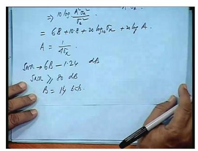
You also saw that SNR signal to noise ratio in terms of logarithmic ratio is 10 log sigma x squared by sigma e square, if you write this, if It is amplified by a factor A, that is A into x n is the output then variance will be a square sigma x square. So, this sigma x square will be replace by a square sigma x square, if there is an amplification by A. So, that gives me that approximately 6 B plus 10.8 plus 20 log of sigma x plus 20 log of A, if A is 1 by 4 sigma x.
