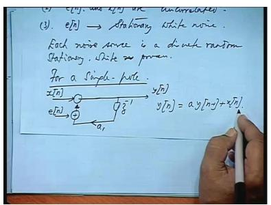
And variance will be 2 to the power minus 2 B by 12, where the same logic, then the error sequence has got no bearing with the input. So, error sequence e n and x n are uncorrelated, again error sequence is random and it is a white noise process. It is stationary, when do you call a sequence stationary, when the statistics that is the first moment, second moment, they are all constant.
