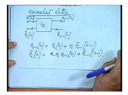
So, the magnitude of K i is must be less than 1 for an all pole realization, there are some interesting simplifications of this let us consider a normalized lattice, if you write this is the lattice block the inputs and outputs in pairs. So, this is e i n, e i n, this is e i tilde n, this is e i minus 1 tilde n and this is e i minus 1 n, so this is the i th block, e i minus 1 n is equal to e i n plus K i e i minus 1 n minus 1.
