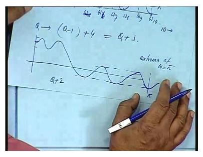
So, Q minus 1 plus 4 extreme that will be the maximum possible number of alternations you can have. So it will be Q plus 3. So, at least Q plus 2 means at the most Q plus 3, is that all right? So, let us sketch one or two more possibilities. This is extra ripple case where we have 10 such alternations.
