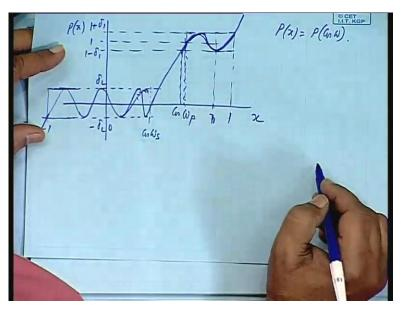
This is x, this is P x. What will be the P x value? P x is cosine omega, all right. P x is basically P cosine omega minus 1, 0. This is cosine omega s stop band. We are assuming that omega s is such that its value is positive; it could have been negative also, then pause band okay, then cosine 0 is 1. This is cosine omega p. This is 1 plus delta 1, 1 minus delta 1, this is delta 2 minus delta 2, all right.
