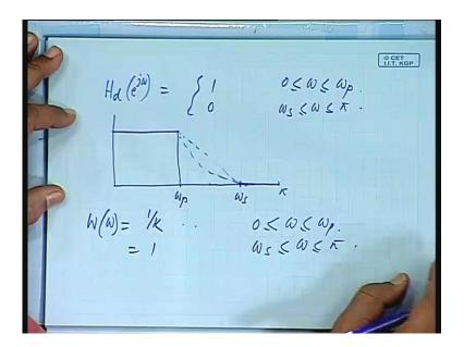
H d is equal to 1 and 0 between omega s and pi, this is the desired response. Like this, it should be it can be like this. We are not putting in this error function, we are not putting any condition here; that means this function will be quantified, this function will be measured only in these two subsets, all right.
