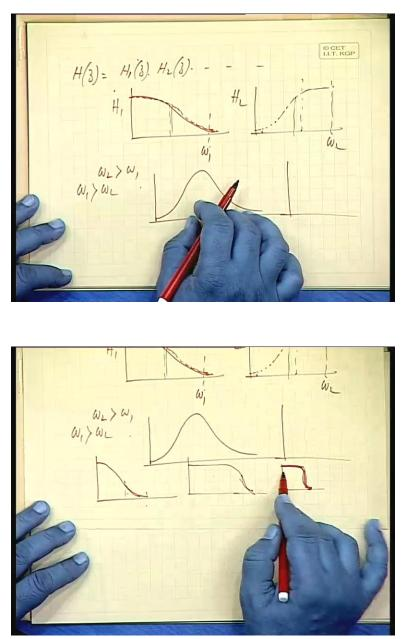
Now, any H z I can always write as, say you can factorize the numerator and factorize the denominator; so H 1 z into H 2 z into so on, so they will be all in cascade. So some may be low pass, some may be high pass and so on. So, it is a net product of all these characteristics that will be determining, the overall characteristics of the function.
