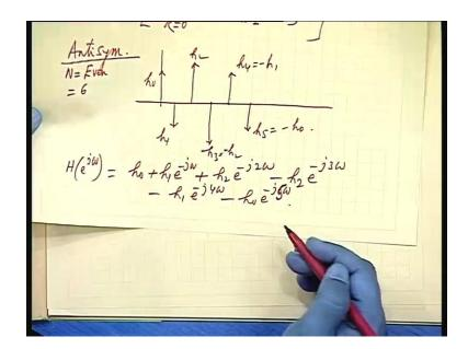
So, it is N minus 1 by 2 omega common, okay. Then 2 into sigma h K, if I write K varying from 0 to 3 that means; N by 2 minus 1, is that all right. N by 2, 8 by 4, 8 by 2, 4 minus 1 3, h K cosine, how much is it? 3.5 means, N by N minus 1 by 2 by 2 minus K into omega, is it all right? So, this is for N even. So, N even and N odd, there will be differing in the general expression; not in this, this is same, phase is same, N minus 1 by 2.
