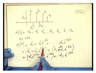
Suppose, we have a symmetric distribution okay h n is a finite length; that is only the numerator, again only the zeros, which is h 0, h 1, h 2, h 3, h 2, h 1, h 0 that means. Suppose, h 0 is this much, h 0, h 1, h 2, h 3 then again h 2, that means h 4 is h 2, h 5 is h 1, then h 0. How many points are there? One, two, three, four, five, six, seven, so number of points N is odd, okay.
