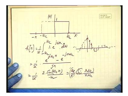
Suppose, you take a very simple function like this; it is already defined here also because it will be a mirror image. So, minus p i to plus p i and this is the cut off omega c, minus omega c. I am
