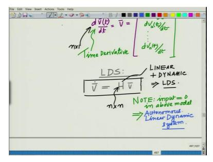
So, this is the time derivative and essentially the linear dynamical system the LDS can be characterized as v bar dot equals H times v bar. This is the fundamental equation of the LDS that is the time derivative v bar dot is a linear transformation of the output is H. This is a matrix H times v bar. So, this matrix H is naturally a square matrix. This is an N cross N because this is also N cross 1 vector.
