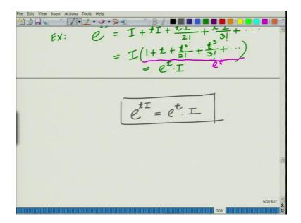
This is termed as recognize this is e raised to the power of a matrix, e raised to the power of t times H. We have not seen this before. This is known as a matrix exponential. This is a very interesting definition. This is a matrix exponential and the way it is defined is, you know the power series e x equals 1 over 1 plus x plus x squared over 2 factorial plus x cubed over 3 factorial plus so on and so forth.
