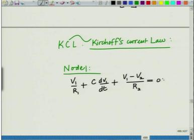
Nodel:  $\frac{V_1}{R_1} + \frac{C}{dt} \frac{dV_1}{dt} + \frac{V_1 - V_2}{R_2} = 0$  $\Rightarrow \frac{dV_1}{dt} = \frac{-V_1}{C_1} \left( \frac{1}{R_1} + \frac{1}{R_2} \right) + \frac{V_2}{C_1 R_2}$  $\Rightarrow V_1 = \frac{-V_1}{C_1} \left( \frac{1}{R_1} + \frac{1}{R_2} \right) + \frac{V_2}{C_1 R_2}$
