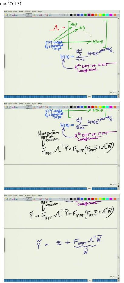
Therefore, it is easy to invert. Remember lambda, if you look at, if you recall the structure of lambda; this basically contains simply your DFT coefficients of the channel taps. So, these are basically the DFT coefficients or these are your FFT coefficients of the channel taps and we also saw what we mean by H k. H k equals summation n equal to 0 to capital N minus 1, h n e raised to minus j 2 pi n k over N.
