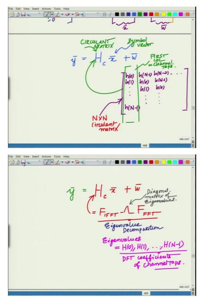
And therefore, I can represent this as y bar equal to H c, x bar plus W bar this is your symbol vector and this is your circulant matrix. Hopefully all of you remember that this circulant matrix is basically one in which each successive column or each successive row is obtained by circularly shifting the previous row or column.
