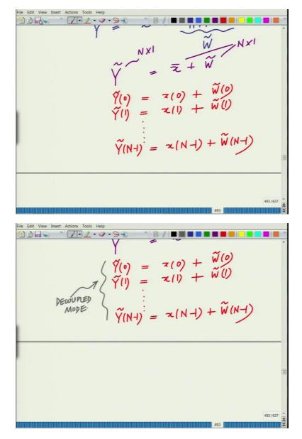
So, essentially what you will have is now after the IFFT, you will have Y Tilda which is basically your N cross 1 vector, equals x bar plus W Tilda where both of these are also naturally N cross 1 vectors and therefore, what this essentially means is now, you have a very simple model Y Tilda 0 equals x of 0 plus W Tilda 0, Y Tilda 1 equals x of 1 plus W Tilda 1 Y Tilda N minus 1 equals x of N minus 1 plus W Tilda N minus 1.
