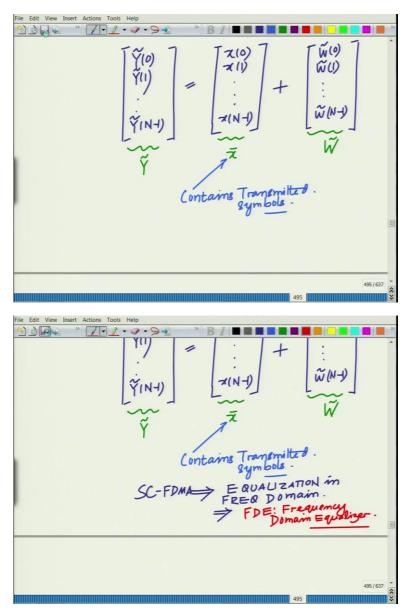
So SC – FDMA, hardware complexity is much lower because low PAPR, because of the low PAPR. So, hardware complexity is much lower and as we have seen the overall system model is basically after the IFFT, you will have Y Tilda 0, Y Tilda 1, Y Tilda N minus 1. This is equal to your x of 0, x of 1, x of N minus 1 plus you will have your W Tilda 0, W Tilda 1 up to W Tilda N minus 1.
