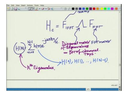
So we have the OFDM, Orthogonal Frequency Division Multiplexing, so we have the OFDM system model that is y bar equal to H c times x bar plus W bar this of course is the noise. We will not dwell upon this too much except to realize that noise is a very important aspect of any communication system. So this if you look at this vector, this is y 0, y 1, y N minus 1.
