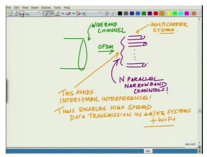
So essentially if you look at this schematically, what is happening is you have this OFDM you have this wideband channel and what OFDM does is takes this wideband channel, converts it into N parallel, splits this into N parallel, OFDM splits this into N parallel narrowband channels that is essentially so the data rate, effective data rate is going to be the same, but the second system is much more tractable.
