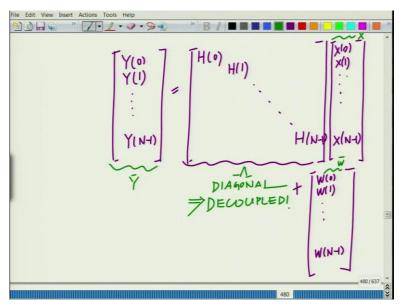
So, if you write this you will have then, if you write this you will have then Y 0, Y 1 up to Y N minus 1. This is equal to the diagonal matrix H 0, H 1 up to H N minus 1 times X 0, X 1 up to X N minus 1 plus your noise which is W 0, W 1 up to W N minus 1 and because this is a diagonal matrix, remember this is nothing but your diagonal matrix, this is your lambda.
