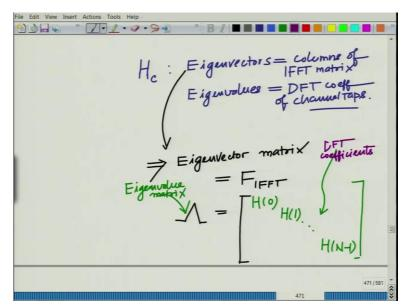
So, H c has the following very interesting property. H c Eigen vectors equals columns of IFFT matrix and Eigen values equals the DFT coefficient. Eigen values are the DFT coefficients of the channel taps and this also implies that the Eigen value matrix, implies the Eigen value matrix if you look Eigen value matrix, this is equal to simply the column of the matrix which contains the IFFT columns of the IFFT matrix.
