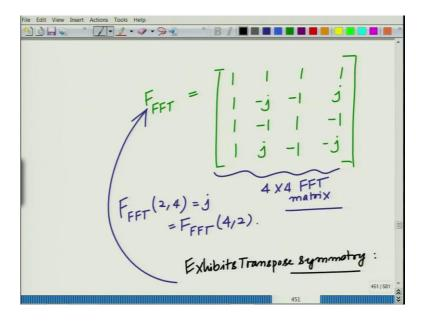
So, you will get F FFT this is the 4 cross 4 matrix this will be equal to 1 1 1 1 1 1 1 1 1 this will be W which is minus j W square which is minus 1 W cube which is j W square which is minus 1 W four which is 1 W raised to six which is minus 1 this will be W raised to W three which is j this will be W six which is minus 1 and finally we have W nine which is minus j and this is the Fourier matrix this is a 4 cross 4 Fourier matrix.
