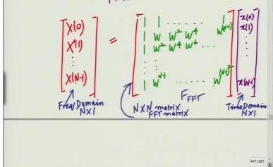
And now, the linear algebra part now FFT and IFFT can be represented FFT operations and IFFT operations can be represented as matrices or rather you can say matrix transformations or linear transformations so, these are nothing but, linear transformations, what are these linear transformations?
