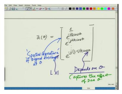
And you can see this a bar of theta this has an interesting structure, let me just write this again over here, this has a graded phase constant phase offset of e raise to minus j k cosine theta with respect to e raise to minus j k cosine theta e raise to minus j 2 k cosine theta, e raise to minus j L minus 1. So, this depends on theta as you can see, this is an L cross 1 vector and this is it depends on theta.
