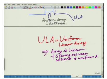
ULA stands for and this is very important concept in signal processing, ULA stands for a Uniform Linear Array implies, which essentially implies that array is linear plus spacing between antennas is uniform which is equal to d, the spacing between the antenna antennas is equal to d.
