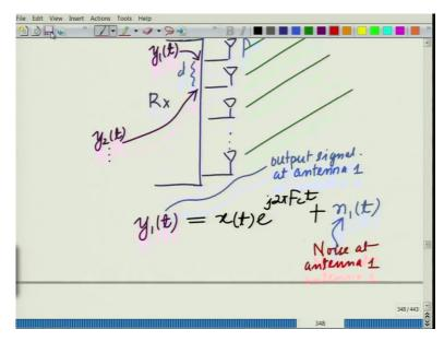
So, you have the antenna array and you have the signal that is arriving at an angle of theta and this is the distance between the antenna elements d and this is the signal x t, you can say this is x t into e raise to j 2 pi. This is the signal at the first antenna element that is x t into e raise to j 2 pi fct. So, we have y t So, the signal at the first antenna is we can write this as y t or y 1 t if I recall that as the signal arriving as the output signal at the first antenna. So, this is
