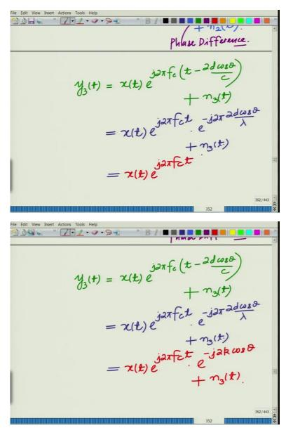
And similarly, so essentially, we are using the property that where you have the signal received at the second antenna is a delayed version of the signal received at the first antenna.
