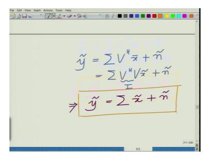
Now, you substitute this in our model that we have over here, that is, you have y tilde equals Sigma V Hermitian x bar plus, n tilde. You substitute the model, the pre-coding model, that is, V Hermitian V times x tilde plus n tilde and V Hermitian V is Identity, so this gives us, this implies, we are left with the model, this reduces to y tilde equals to y tilde equals to Sigma times x tilde plus n tilde. And this is very interesting. Why is this interesting?
