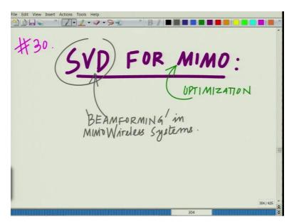
So let us look at SVD specifically for MIMO systems and how SVD helps in the optimization. We are going to eventually look at a very important part of MIMO optimization. In fact, SVD is used for Beam Forming, the idea is that SVD, this can be employed for what we call as Beam Forming, as we have looked at in several times, that is, Beam Forming in wireless systems, especially MIMO wireless systems.
