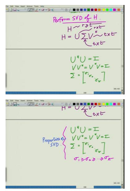
So we perform, we start by performing, in this journey of obtaining a decoupled system, we start by performing the SVD, singular value decomposition of the channel matrix H. And let us again consider a system with r greater than equal to t, number of receive antennas greater than equal to number of transmit antennas.
