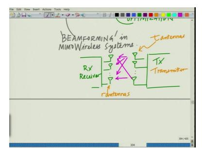
Let us again look at a typical MIMO system, which is basically, has multiple antennas at the receiver and multiple antennas at the transmitter. So you have the receiver, you have the transmitter, you have r antennas at the receiver, t antennas at the transmitter and then you have the channel coefficients where we know that we have the channel matrix. H denotes the channel matrix.
