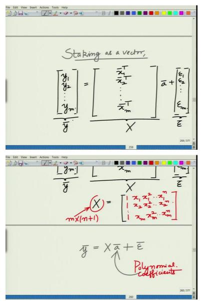
And now, again staking these as a vector, the vector model can be developed as we have y1, y2, yn or rather y1, y2, ym. This is equal to x1 bar transpose, x2 bar transpose, xm bar transpose times a bar plus you have the errors epsilon 1, epsilon 2, up to epsilon m. So, this is x, this is y bar and if you look at the matrix X, this has an interesting structure.
