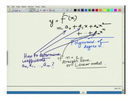
That is we want to approximate y as f hat of x, which is essentially a naught plus a1x plus a2x square plus so on an x raise to the power of n. So, this is your polynomial of degree n. So, this is the polynomial, nth order of polynomial or polynomial of degree n. So, how do we develop and of course, now, if n equals to 1, if the degree is 1, then it becomes a linear fit, which is what we have already seen in the linear regression.
