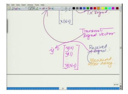
And let us say this is your  $\overline{y}$ , which is a reflected signal. Again, you have the samples of the reflected signal or the received signal. You are transmitting a signal from the RADAR and you are measuring the response at the radar after a certain delay. So, this is your received signal which is measured after a certain delay.
