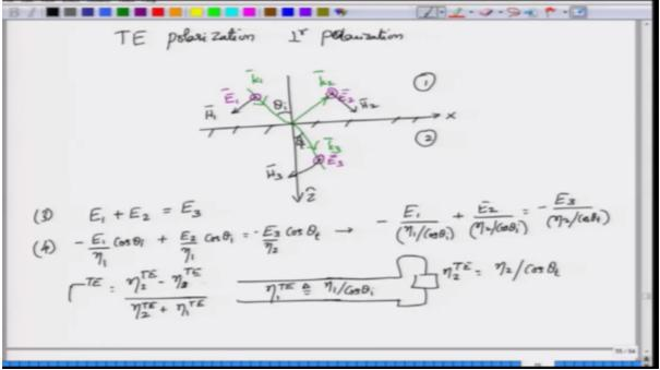
So solving for this  $\Gamma^{\text{TE}}$  or equivalently  $\Gamma^{\text{TE}}$  from these set of questions is as simple as writing down the appropriate reflection coefficient expression for the transmission line case. A longer calculation indeed confirms that what we have written is true. Okay.
