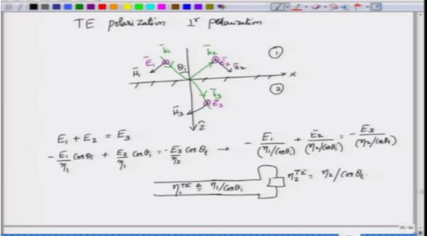
Of course,  $\theta_i$  and  $\theta_t$  are still related in the same manner as Snell's law, so there is no change. So what you should understand is that this scenario of TE polarisation can be made exactly analogous to a transmission line that we have already seen with the impedances being  $\eta_1^{TE}$  for the main transmission line. That transmission line is terminated in the load whose impedance is  $\eta_2^{TE}$ .
