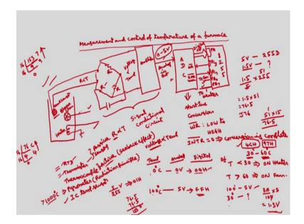
Suppose if I want to measure and control the temperature of a furnace, measurement and control of temperature of a furnace. Suppose I have furnace here, here you have to insert a sensor temperature sensor, this is temperature sensor and here we can control this temperature maintain the temperature by using a fan and blower and heater.
