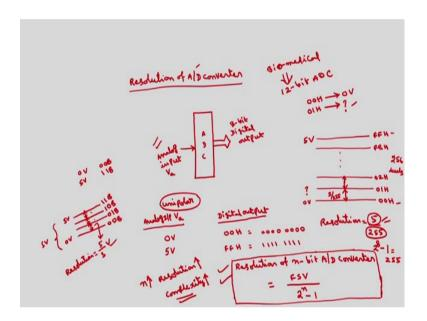
How to define the resolution of A to D converter? So, if you take the A to D converter analog input voltage output is digital. If, you take unipolar A to D converter, in case of unipolar, this analog value Va if I assume that Va and digital output; if I assume that 8 bit digital output, digital output, analog input. So, as the name implies unipolar, we have only one single polarity means all positive voltages only.
