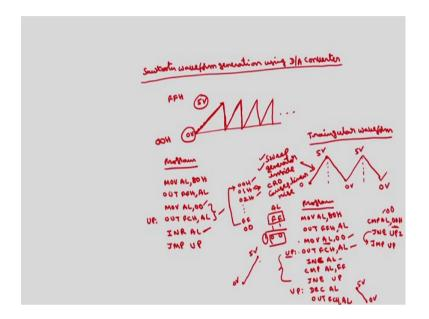
So, how to generate a sawtooth wave form? Sawtooth waveform generation using D to A converter, sawtooth wave form is nothing but how to I mean change from one level to if I start with 0 volts and if I take the peak value as 5 volts. So, it has to I mean rise in a linear fashion from 0 volts to 5 volts and then it has to suddenly drop to this is the x axis suddenly drop to 0 volts, again it has to rise from 0 to 5. So, only drop to 0, 0 to 5, 0, 0 to 5, 0 and so on.
