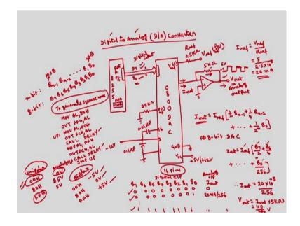
So, if I take here 8255, I will connect to port A of 8255. So, using this 8255 I can give these values accordingly we will get the proportional current proportional voltage here. Now suppose if I want to I mean generate square wave if I connect this Vout to this CRO. So, I want to generate here square wave with the voltage of 0 volts and 5 volts.
