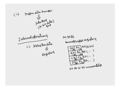
Then the third operation will be-perform the data transfer. So, this will be performed by a data bus. So, in case of 8086 we have 16-bit data bus. So, in order to perform the very first operation which is microprocessor initiated operations; such as memory read, memory write, IO read, IO write. So, we need address bus, we need some control signals, we need some data bus. So, finally, after discussing about all these operations I will draw the overall architecture of 8086.
