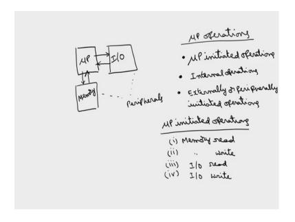
So, the block diagram of this microcontroller; as I have told this is microprocessor IO and memory. This IO and memory are called peripherals. Without this memory and IO, the microprocessor cannot perform any function. Now, this is you have to I mean connect memory to the microprocessor. The technical work used to connect this memory to microprocessor is called interfacing.
