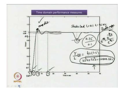
We can see that the closed loop response of the system is obtained as shown over here where we have got the overshoot undershoot before settling down. The output has got overshoot, undershoot, overshoot little bit of undershoot over here, before settling down to the reference value. Similarly, when a static load disturbance of magnitude load of magnitude 1 equal to 0.1 is applied at time T equal to 35 second, we have got the disturbance response in this session.
