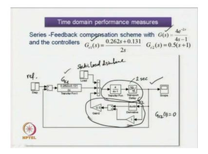
Let us consider the block diagram shown over here. This block diagram shows us a Series Feedback compensation scheme where we have got a controller GC 1 in the feed forward path and a controller GC 2 in the Feedback path, thus we bring us a series feedback compensation scheme.
