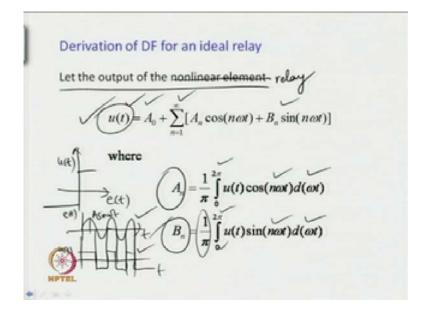
So, the equivalent gain of the relay is given by 4 h upon pi A. The equivalent gain of the relay is derived as 4 h upon pi A. How we have obtained that one we shall discuss in detail.
