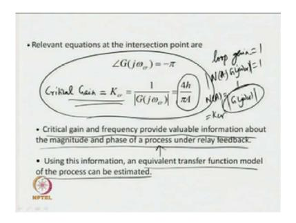
What more we can get using the Nyquist plot, we can get some simple expressions. Now, the phase of the process at the critical frequency will be equal to minus pi; why that is so? If we consider the loop gain, loop phase also we know that loop phase is equal to minus pi. In this case, what we have in the loop? N A G s as the loop gain, which in frequency domain gives us N A G j omega; at the critical frequency, the loop gain will be N A G j omega c r. So, this phase will be equal to minus pi.
