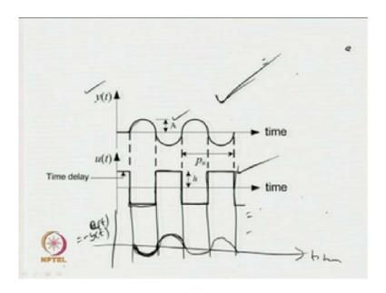
The output can assume this form (Refer Slide Time: 11:08). So, let the output of the autonomous relay control system be shown as like here. So, y t versus time t is given, where the oscillation starts from here and we have got sustained oscillatory output of this form.
