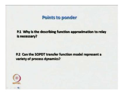
Points to ponder: first point could be like this, why is the describing function approximation to relay is necessary? It is easier to estimate the unknown parameters of an assume transfer function model with relative each, when the relay is described by an equivalent gain, when the relay dynamics is available in the form of equivalent gain.
