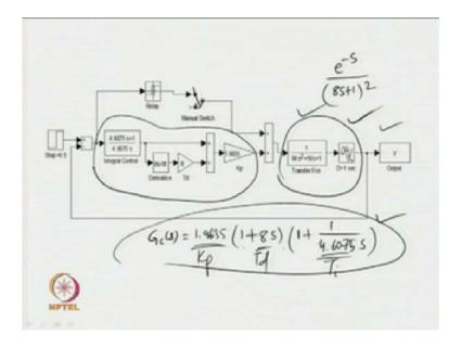
Now, let us come to this simulation diagram. So, in this simulation diagram we have considered a second order process dynamics which is given by e to the power minus s upon 8 s plus 1 square. Now, the process is connected to a series PID controller; the series PID controller is given as, G c s is equal to 1.9635 times (1 plus 8 s) times (1 plus 1 upon 4.6075s). So, the process has been subjected to a PID, series PID controller.
