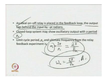
Next, some characteristics of relays will be studied. What we have done? An ideal on-off relay is placed in the feedback loop then, the output lags behind the input by pi radians. So, the relay is forcing, this relay is forcing (Refer Slide Time: 15:11), the planned output to be of sustained oscillatory and that relay is also introducing a phase lack of
