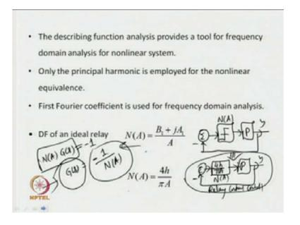
Let me go to this page and let me explain. So, we have got the autonomous relay control system given by a summer; then we have got the relay over here, then we have got the process, then output and negative feedback. These can equivalently be represented by an autonomous loop with the gain of 4 h by pi A, p, y. So, this equivalent closed loop transfer closed loop system very much looks like the closed loop system, we had with a proportional controller.
