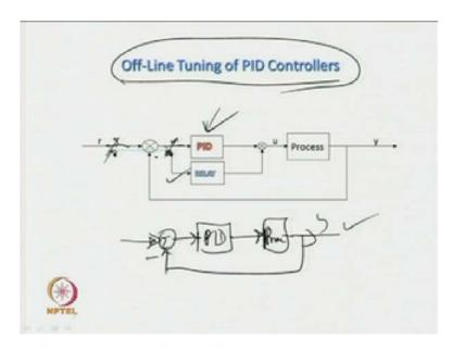
Let us consider, a relay control system of this form, where we have a PID controller, a controller in the PID forward path and a relay also there in the PID forward path; whereas, we have got two switches, one switch over here and another switch over here (Refer Slide Time: 01:03). When the switches are down, then the relay gets connected to the process and we have got relay and process in the closed loop system.
