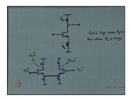
So, for example, the common source amplifier you remember right. So, ordinarily the common source amplifier the source is at ground, but let us have a resistor at the source in which case this becomes the source degenerated common source amplifier.
