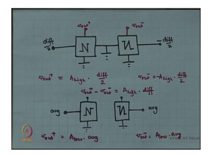
Now, let us do them; so, my first experiment is going to be diff by 2 and diff minus diff by 2. And when I do this node is at ground we know that that node is a ground which means that v out plus. So, now these two networks are decoupled from each other because the middle is at ground. So, they are really not coupled to each other anymore, but they are identical otherwise.
