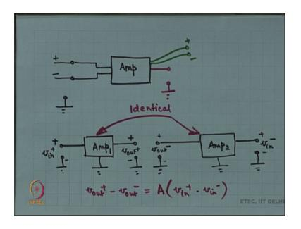
So, invariably your input signal to your electronic system is the difference of 2 potentials as opposed to an absolute potential with respect to ground alright; this is basically what is going to happen in future.
