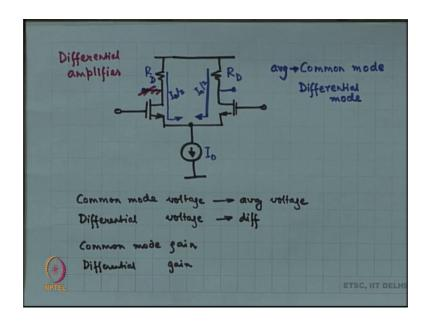
And draw it like this now when you have placed the current source over there automatically the DC operating point is also established for example, if this is I naught and these two are perfectly symmetric R D and R D. Then I naught by 2 is going to come through each MOSFET right and you have established the current through each MOSFET. So, all of these are falling into place.
