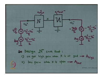
So, I am going to apply v in plus over here and v in minus over here right and I can always think of v in plus and v in minus as the superposition of 2 voltages; One being the difference of the 2 and the other being the average of the 2 right. Likewise v in minus is equal to minus v in plus minus v in minus by 2 plus v in plus plus v in minus by 2.
