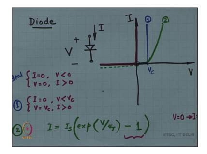
And this we will start from the symbol of the diode ok. So, diode is made out of a p-n junction all of that is there we are going to bother about it; however, if the current through a diode is I and the voltage across it is V; then V and I have a certain graph what does that graph look like? Do you know? I am sure you know that.
