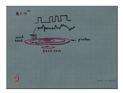
I do not know if you have seen the insides of the hard drive, but his flatter and if you think of a 1 terabyte hard drive; it has 1 kilo means 1000 mega is a million, Giga is a billion, Tera is a trillion, right. So, 1 terabyte refers to 1 trillion bytes. So, 1 trillion bytes 1 into 10 power 12 bytes and each byte is made up of 8 bits stuff that you know already.
