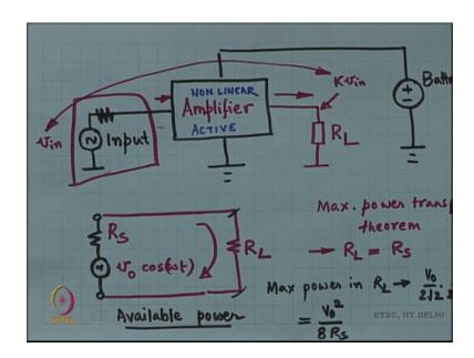
So, what we normally have think of in is a black box; think of a black box and in this black box I am willing to give you extra power from a battery ok. There is a battery take as much power as you want from the battery. Now I am going to give you an input; so, here I am showing a sinusoidal voltage source, but this is really a sensor right and when we say that it is a sensor, the sensor is going to have to some source resistance.
