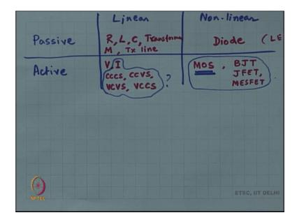
So can you fill up this table linear passive components are what? R, L, C, transformer, mutual inductance right these are all linear and passive. So, transmission line these are all linear and passive elements non-linear passive elements; give me an example, diode great; active? Linear active elements do you know any elements that are linear and active? Example, voltage source ok, current source these are 2 main things right.
