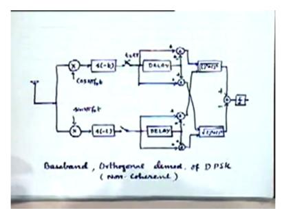
And keeping that view in mind we arrive at a receiver structure which is essentially that of that base on the concept of de-modulation of orthogonal waveforms right, this was the receiver structure that we looked at.
