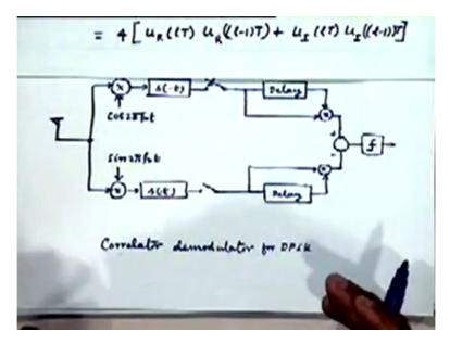
That brings me to this kind of a receiver structure, this is a receiver structure that is implied, it is really so simple. You are taking Ur LT you see what I have doing, you are taking Ur LT and multiplying it with a delayed version of the same thing right, so this is your LT and multiplying now you are not adding or subtracting you are multiplying the two right. Similarly you are taking U I LT and multiplying with a delayed version of the same thing and subtracting the difference right.
