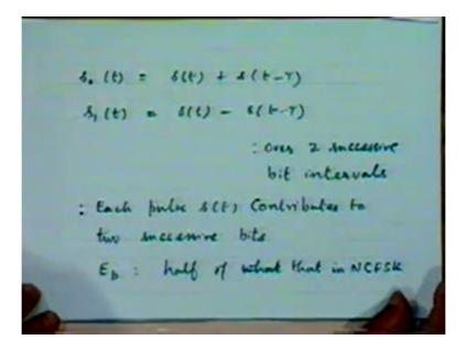
So the energy is double which is what I want to say here that each pulse each individual pulse S t contributes to two successive bits, therefore if you want a given performance the energy in individual bit interval could be half as much right.
