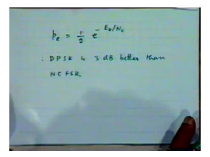
So we already have the expression for the performance of non-coherent FSK we just derived it to a morning, that was half of minus Eb by 2 N0, so now it will become Eb by N0 right. So that is the conclusion DPSK is about 3 dB better than non-coherent FSK, is argument clear?
