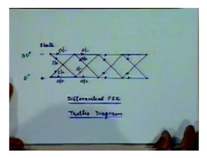
So that is how you do, zero implies no phase transition, one implies (a phase) offcourse could be the other way around without any, you could express this also in terms of a trellis diagram, were the straights are the polarity whether it is negative polarity or plus or it could be zero degree phase or this could be lets say if this is negative we could say 180 degrees this is zero degree right.
