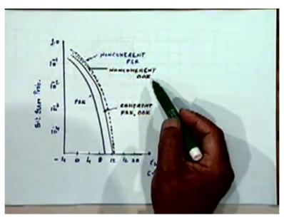
This black dotted curve is what you get for non-coherent On Off Keying ok. Now noncoherent On Off Keying is we already seen it is not very good because it waste 3 dB of power
