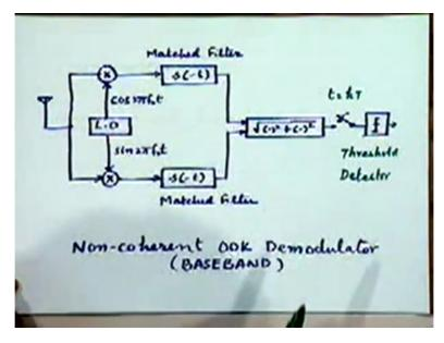
If you remember your non-coherent On Off Keying receiver was something like this at the baseband right, that is you have the baseband output coming out of the I Q de-modulators right and we are assuming that your transmitted signal is A times S t right or it is either there or not there, either with amplitude A or with amplitude 0.
