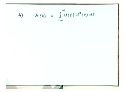
Because suppose (we are) our designated sampling instant is t equal to 0 then we have appreciated before we try to discuss that several times that this value R sub 0 R of 0 is nothing but the correlation of the received signal with the transmitted signal right.
