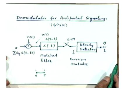
So to start with let me discuss this picture for the de-modulation for antipodal signals. So I am taking the case of an antipodal signals here of which BPSK is an example binary phase shift key is the main example of antipodal signaling in more spectacle applications.
