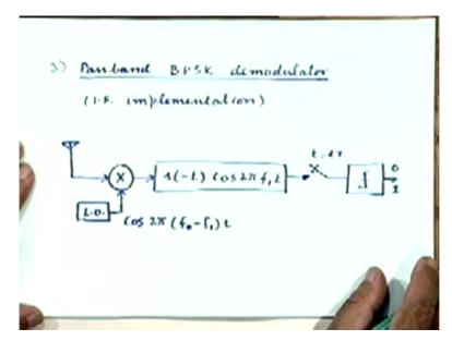
So this is an alternative passband BPSK de-modulator which is the same as before except that instead of a match filter being matched to S minus t cosine 2 Pie F1 t, F0 t it is matched to some other frequency F1 t which is an intermediate frequency of operation.
