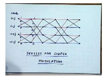
And in the digital modulation context it is conventional to represent this finite state machine action by means of a diagram called the trellis diagram so I am going to introduce to you what is a trellis diagram the concept of it trellis diagram, this is a trellis diagram for OQPSK modulation now first what is a trellis diagram basically a trellis diagram consist of a set of loads which represents that different possible states in which your machine can be right.
