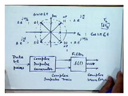
And this was the picture that I think I showed you at that time this constellation diagram corresponds to QPSK to recapitulate for you we have two quadrature carriers in QPSK, each modulated by possibly one or the two bits that either we can think of these two carriers being independently modulated by two streams, two bit streams or on a block basis that is we take two bits at a time and use one of this points as a signal for representation of those two bits.
