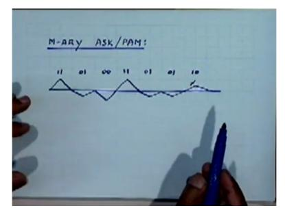
An example here of a waveform, a 4-ary waveform corresponding to M-ary ASK where just for the sake of illustration chosen a triangular pulse a four possible different amplitudes right, this is one amplitude, this is another, a third and a fourth, these are the 4 amplitudes that are coming up and we have associated with each of these amplitudes a binary sequence of length 2 right so when the two successive bits are 1 1 maybe you transmit this amplitude 0 1 this amplitude so on okay.
