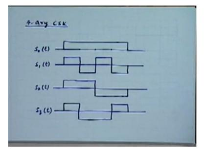
Yet another example of orthogonal set of waveforms is a set of pulses like this right as you can see if you were to multiply them out and integrate the result they will be, the integral will turn out to be 0 any pair of them right and this is called 4-ary code shift keying C is standing for code okay so basically we have a different code for representing each waveform different binary code right.
