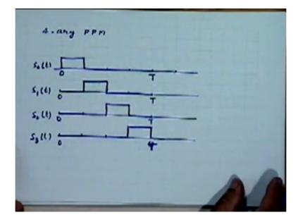
So anyway I thought since that point came up for discussion last time which I could not satisfactorily address I should have at least point this out to you at this point, so this is one example of orthogonal signalling, here is another example of orthogonal signalling, very simple trivial kind of example so here is your S o t which is the waveform is to be regarded off duration T upto here it starts here and ends here right.
