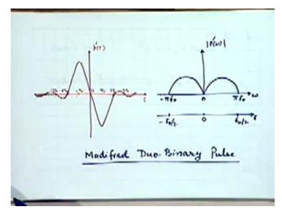
Okay I will have to fill them out of my hat here again, which waveform you would like to look at? The modified duo binary, this is the modified duo binary waveform right, now of course if you remember realization with which you are working as the delay of 2 T0 seconds right because what we are saying is, we are sampling at every T0 seconds, so what you have to really see is if you were to super impose this waveforms one after another every T0 seconds right, what will happen?
