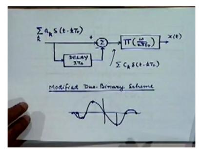
Modified duo binary scheme is in which you have right, sampled values that come to the picture is this, this and this, non-zero sample values okay all others after that will go through zeroes right here, here, here later on it will be all zeroes, ya so I am talking about these three although it is 0, since it lies within the span of non-zero values I am counting it as, I am denoting it by f, some value right some notation yes.
