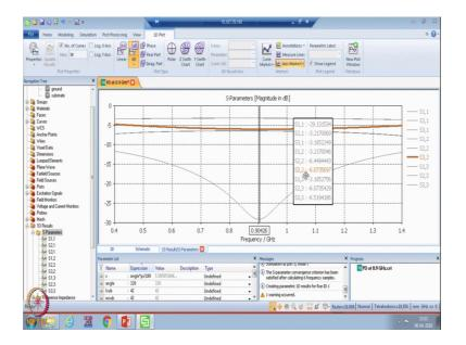
So, now it has been simulated, just to check the response, here you can see. So, this is S1, 1 this red one. So, you can see it is below 10 dB in all the frequency range from 0.4 to 1.4 gigahertz, and at 0.9 gigahertz it is resonating. Now, if we see S2, 1, and just try to locate the marker using this option, axis marker. Now, if you read the value of S2, 1, it is minus 3.21. So, ideally if there were no losses in the substrate, it should be minus 3 dB, but since the substrate is lossy.
