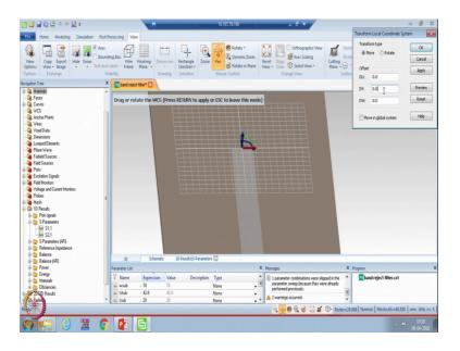
Now, we will try to design band pass filter. So, to do that just go to modeling, select this edge align WCS. And then just give a offset, because you want to put a via over here. So, give some offset for local coordinate system. So, use transform, and now so you need to transform in V by some x parameter. Let us take x as around maybe 1 mm.
