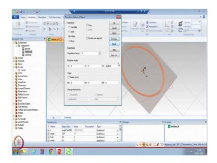
Then select rotate, and then in W you give angle by 2. So, now it has rotated, then press ok.
