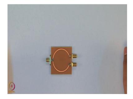
Now, we will try to design a two way power divider. So, this is a PCB for two way power divider, it is made on FR-4 substrate, whose thickness is 0.8 mm. Here, this is input port, and these two are output ports. So, you can name it as port 1, 2 and 3. So, if a power of 1 milli watt is given at port 1, you will get half of the power at port 2, and half of the power at port 3.
