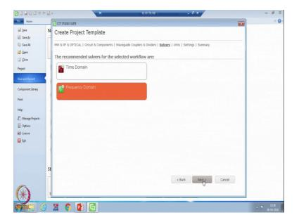
And this time, we will do the simulation in frequency domain. Last time, I did the simulation using time domain method, this time we will use frequency domain method. So, I have selected frequency domain.
