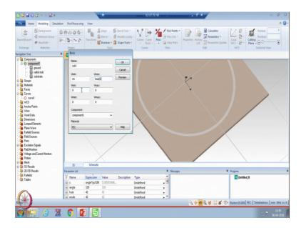
Now, if you see, it is aligned with the coordinate system. Now, we need to make the ports. So, to make port again select brick, define ports, so maybe just take as output 1. And if you see now, you try to make it from here. So, just make a strip from this end to this end. So, this is rin, and outer will be 1 sub by 2 ok. And for V this should be 50 ohm strip. So, for FR-4 substrate with 0.8 thickness, the w is 1.5 mm. So, for the time being
