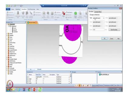
So, you have made the port you have made the geometry, next you need to do the simulation. So, to do the simulation go to simulation, again go to frequency setup solver. Before this, you need to give the settings, here you give the frequency range, if you have not defined it earlier, give it from 0.4 to 1.4, and then boundaries. Use open add space in all the planes, and then simulate it using frequency domain solver. Now, just wait for its response.
