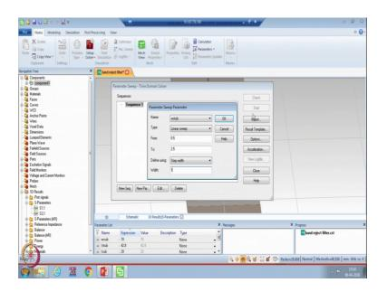
Now, go to parameter sweep, select first new sequence, then you select new parameter. Now, I want to change the width of the stub, because I want to see the behavior of the stub width. So, I will select wstub, and this range is 0.5. So, just to see, I will change this width from zero point to 2.5 in the step of 1 mm. So, I have given here 1 mm step width, and then press.
