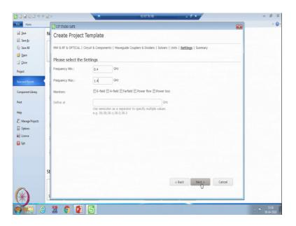
So, we will select the frequency range from 0.4 to 1.4 gigahertz, so that the center frequency will be around 0.9, and it will come in this particular range.
