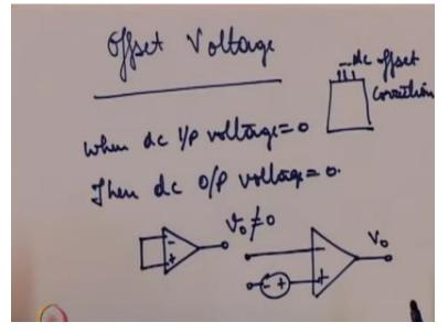
We call in the first lecture I had mentioned that when you have a fan chip, there are some pins allotted for dc offset correction, so this correction is related to this concept of offset voltage. Now ideally when dc input voltage = 0 then dc output voltage should also be = 0, so in other words if we have an opamp connected like this Vo should be = 0 but in reality, this is not see this is what is known as offset voltage.
