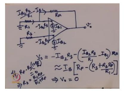
Now to get rid of this what can be done is we can introduce a resistance R3 in series with the non inverting input, so we have so the current flowing here is IB2 the voltage here is -IB2 R3 if the voltage is -IB2 R3 then it must be -IB2 R3 here as well the current flowing here is the current flowing here is the current flowing through this -IB1 so therefore the current flowing is IB2R3 upon R1- IB1.
