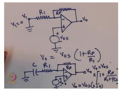
Or even if suppose this we ground so V1 = 0 then what happens is that Vo is simply = Vos 1+ this is Vos is in the non inverting configuration so we have an output voltage which is like this and the problem is that this Vos is now amplified by this factor easy solution of this is of course to have some internal circuitry within the opamp to correct this input voltage.
