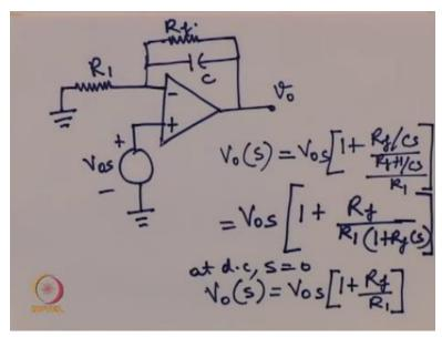
So to alleviate this problem or to at least ensure that output does not keep increasing linearly with time what is done is that if we have a resistance in shunt with the capacitor like this and by the way usually most capacitances have a certain Rf resistance in shunt so we do not always have to explicitly add this resistance, so then what happens the Vos that is the output voltage it has an expression like this okay and this can be simplified to Vos 1+Rf upon R1 1+RfCS
