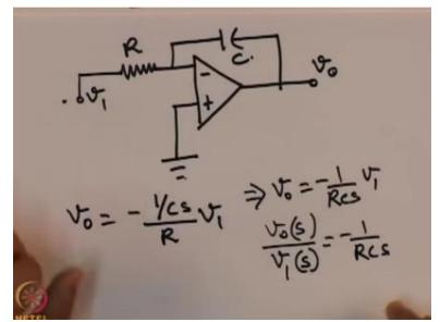
Of course, we can simply analyze this as v0 is equal to -1 upon CS upon R v1 which implies v0 is equal to 1 upon Rcx v1 now this is a low pass transfer function, if we can write a transfer function of the system it is v0 upon vs 1 upon Rcx, as we can see this is a low pass transfer function, because as s tends to infinity the value of the magnitude of this transfer function keeps decreasing, but in order to also see the time domain response let us try to write the time domain equations.
