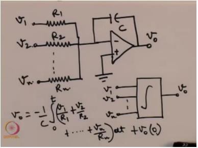
So this is the block diagram of this integrator or summer integrator and the output Voltage in time domain is given as you where this v0 at 0 is the initial condition so this is the formula for integrator now just like the non-inverting or the inverting amplifier we also have to take into account the currents that are flowing so just like the previous case suppose we have a limitation on the maximum current that can be supplied.
