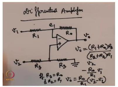
So here this is a combination of both the inverting and non-inverting opamp, if only v1 is present and v2 is not present then by virtue of this short this point will also be shortened, which basically means that there is this R3 plays no role because the current here is 0.
