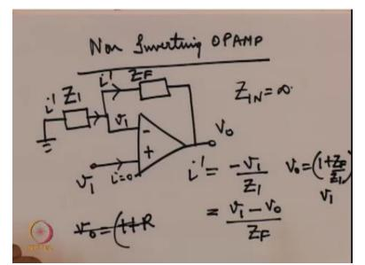
So we had an inverting configuration now we have a non-inverting configuration so the non-inverting configuration so the non-inverting opamp, now let us try to derive the relationship between v1 and v0 again we note that the current flowing in the non-inverting terminal will be 0 because the input impedance of the opamp is very high therefore for a non-inverting opamp Zin will be equal to infinity.
