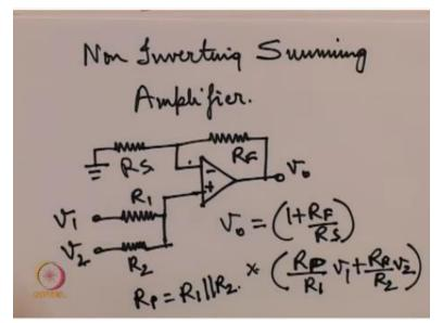
So, we have suppose we have 2 inputs like this we can show that this output V0 will equal to 1+ RF upon RS times R it will be RP this is RP upon R1 times v1+RP upon R2 times V2 where this RP is equal to R1 parallel to R2 in fact for a number of such sources when in here we have considered only 2 inputs.
