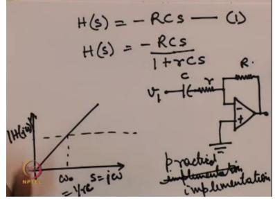
So instead of that, if we have a implementation with a transfer function like this HS, so in this case if I write in our case HS is or the transfer function is equal to Rcs let us label it as equation 1 and if we try to plot this magnitude of HS with omega or we take S equal to J omega and this as H of J omega
