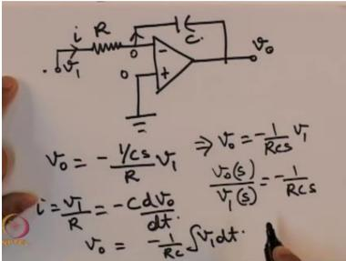
So once again you see that these 2 terminals are at 0 voltage is a virtual short between the inverting and non-inverting terminals and so I can write the current i is again flowing only through i R and C the current i flowing through R can be written as i is equal to v1 upon R and the current flowing through C is -C dvo upon dt.
