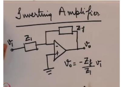
Here we shall be using that formula to further discuss some of the other circuits, so once again if we can write the formula for the general inverting amplifier with general impedances not just resistances, so this is the formulary letting the output voltage v0 to v1 suppose our Z1 and Zf are like this.
