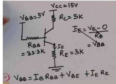
Just like the previous circuit we now have an equivalent voltage source VBB this remains = VCC this is RC this is RE and this is RBB this is = 33.3 kilo ohms VBB is = 5 volts RC is = 5K and RE is = 3K, so now if I want to calculate the individual currents how do I do that VBB is = IV RBB + VBE + IE RE now IB is = IE upon 1 + beta.
