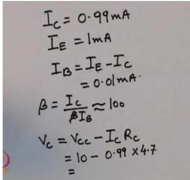
So, I have IC = 0.99 milli ampere IE = 1 milli ampere hence IB will be = IE - IC which is = 0.01 milli ampere, now beta is = IC upon IB sorry IB and that is also verified it is nearly = 100, now if I ask you to find out what is the voltage at the collector terminal VC so VC will be given by VCC - IC times RC which turn out to be = 10 - 0.99 times 4.7 and I leave the evaluation of the final value to you as an exercise.
