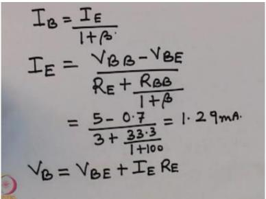
Therefore if I substitute this value of IB into the previous equation okay so I am substituting this value of IB into this equation then what I get is then if I solve for IE what I will get is ok and if I plug in the values then it comes out to be so VBB is 5 volts VBE is 0.7 volts RE is 3 kilo ohms and RBB is 33.3 beta is 100 and this comes out to be = 1.29 milli ampere.
