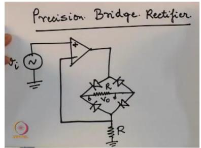
So this is my bridge rectifier circuit, Vo is taken by between these 2 points and I leave it as an exercise to analyze for you to analyze this circuit and show that indeed the threshold voltage problem will not be here and finally we can also find the same, we can also apply the same technique to the peak rectifier circuit that we had discussed earlier.
