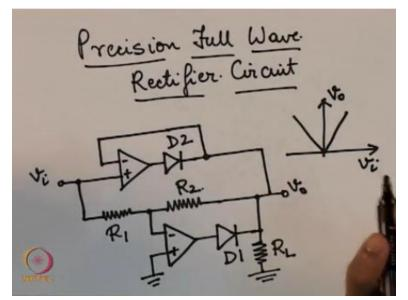
We can all that a precision full wave rectifier circuit so this is just a combination of the 2 this is the first circuit that we had discussed and this is the second circuit we had discussed and the output and input relationship is given by this graph in face, we can obtain a bridge rectifier precision bridge rectifier version of the same circuit also and that is given by.
