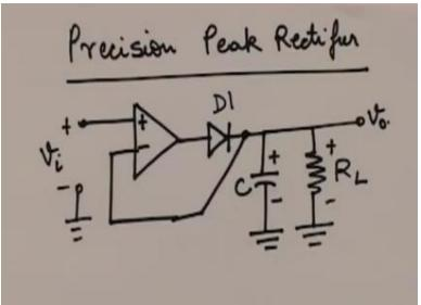
So, this is the circuit for my peak rectifier and again I leave it is as an assignment for you to analyze this you will find the peak the threshold voltage problem is not present in this circuit because of the presence of this op amp, whenever Vi is positive this my this will always be in forward bias mode even for small values of Vi and therefore even for small values of Vi that is when Vi is lesser than the threshold voltage of this diode.
