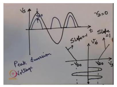
Let me draw the circuit say Vs is positive so then, so this is T this is Vs, so when this is say this voltage is positive Vs is positive then or in the pause or we are in the positive half cycle of Vs this diode D1 will be forward biased and when Vs is above the threshold voltage of D1 this will start conducting when Vs is in the positive half cycle however diode D2 will be reverse biased and will not conduct.
