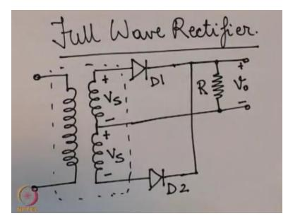
The circuit for that is given like this, so here this part which was not sure not present in the circuit for the half wave rectifier this is actually a transformer this whole thing now the transformer does not really play any role in the rectification, but it is necessary to show it show this element just to just to let you know that there are actually 2 sources + - Vs and + - Vs.
