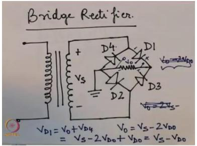
So again, we have a transformer which supplies a voltage of + and - Vs and then we have a bridge circuit, so the bridge circuit consists of 4 diodes connected as shown ok and the principal operation is similar to that of the full wave rectifier see during the positive half cycle this say when Vs is positive then D1 and D2 will be forward biased and during the negative half cycle D3 and D4 will be forward biased, so overall the output input and output relationship will be something like this.
