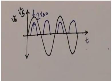
So the shape of the curve is similar to that of the full wave rectifier but the difference between the 2 peaks of the input and output is now = 2VD0 because of the 2 diode drops that we have to
