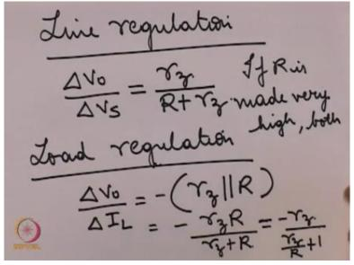
Which is defined as the change in V0 due to change in the source voltage Vs and the other parameter that is also performance parameter of a Zener diode is what is known as load regulation which is the change in V0 due to change in the load current.
