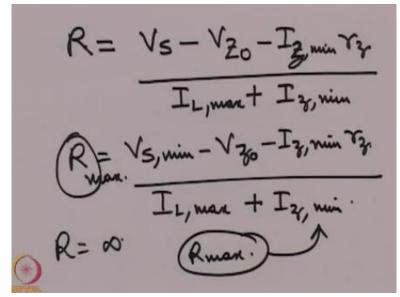
So here I have just substituted in place of I this equation so from here the value of R that we get is =  $VS - VZ0 - IZ \min RZ$  whole upon IL max + IZ min, now suppose there is a minimum value to the supply voltage also so then the value of R will be =  $VS \min - VZ0 - IZ\min RZ$  upon IL max + IZ min.
