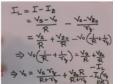
IL is given by this current that is the current from the source and suppose the current through the Zener diode is IZ then IL will be = the difference of I and IZ right now what is this current I can I write this as = VS - V0 ok upon R and what is this current IZ can I write it as V0 - VZ0 upon small rz ok, so then simplifying I get this as = VX upon R okay + VZ0 upon R - V0 into 1 upon R + 1 upon rz okay.
