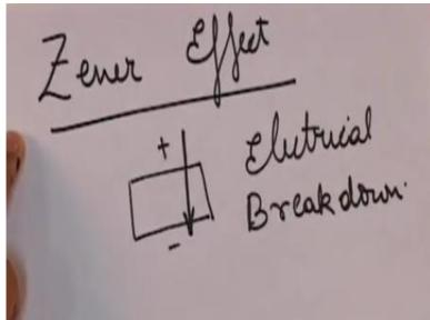
So let us discuss about this Zener effect, first of all we have to understand that the Zener effect is what is known as a quantum effect usually when a material an material is subjected to high voltage at a certain high voltage this will break down means the electrons suppose this was an insulator initially under the influence of the very high voltage the electrons will be pulled out and this material will go from conducting from a non conducting to a conducting
