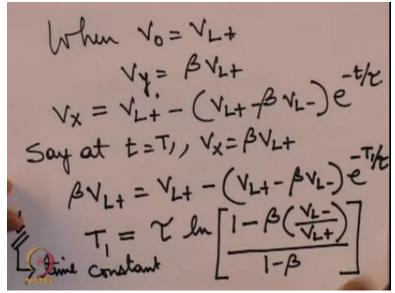
So our if we write it on a fresh sheet Vy is given by Vx is given by ok say at time T1 T = T1 Vx becomes = beta VL+ so then let me substitute that beta L+ is = VL+ - VL+ - beta VL- e raise to - T1 upon tau and the value of T1 if we solve this equation that we should get is like this like this, now here I did not mention what this Tau, Tau is called the time constant for an RC based circuit.
