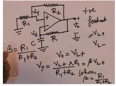
So the circuit for an Astable multi vibrator is like this, this is the circuit again we see the feedback from the output is fed to the non inverting input not to the inverting input so the feedback is positive that is the first thing to know and now in addition to the resistances we also have a capacitance C as you know capacitance is a charge storage element.
