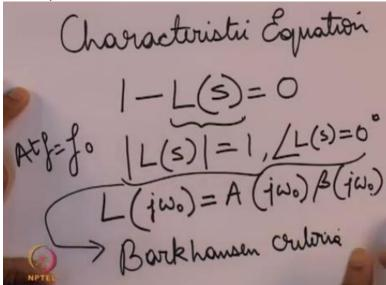
So characteristic equation for this system is given by, So once again the characteristic equation is the denominator polynomial of the transfer function of the system and we had seen earlier that for positive feedback the characteristic equation is given like this, now at a particular frequency say F0 this loop gain the magnitude of this loop gain is = unity so at F = F0.
