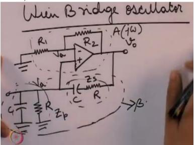
So first let us see the circuit of this oscillator, now in this circuit this part this non inverting opamp comprises the A of J omega part and this part comprises the beta now let us consider suppose the voltage at this point is Va then due to the virtual short affect the voltage at this point will also be VA now if I try to express VA in terms of V0 how will that expression look like, so see VA is obtained from V0 by a simple voltage division because no current flowing inside the opamp.
