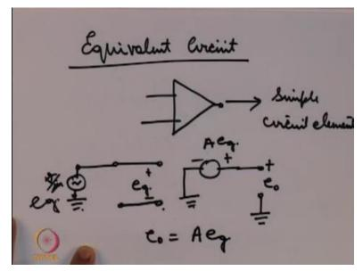
We can draw a simple equivalent diagram so equivalent circuit, now what is an equivalent circuit? An equivalent circuit is a circuit where a somewhat complicated circuit is represented in terms of simple circuit elements it gives a better visualization of this circuit so if you have an opamp the inside of this opamp is like a black box, but if we threw an equivalent circuit we can get a little bit more information about what is going on inside.
