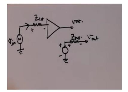
Say, we have an amplifier whose input impedance is given like this, so if you have a source here a voltage source now if Zin is not infinite then there will be a finite current flowing through this input impedance, because of which there will be a voltage drop and therefore at the input of the voltage amplifier the full be in that is the input voltage will not appear conversely for the output impedance.
