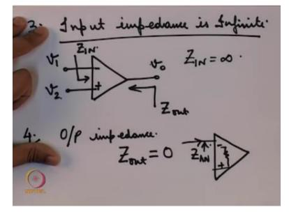
And this now yet another property of the opamp is so once again we have our opamp inverting, non-inverting output. Now if you calculate the input impedance Zin, Zin is always equal to infinity and the fourth point is output impedance that is Z out is equal to 0 now I do not want to delve into the details of this input and output impedance right now but just I will mention that for a voltage amplifier say and how amplifier is a voltage amplifier?
