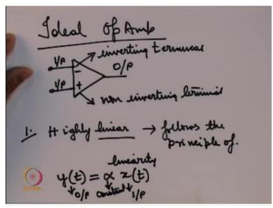
So what is an ideal opamp? An ideal opamp is represented by this circuit, this is the circuit you (()) (03:13) it has three terminals and output and two input terminals, one input terminal is labeled by a minus sign the other input terminal is labeled by a plus sign, the one which is labeled by a minus sign is called an inverting input or the inverting terminal the one labeled by the positive sign is called a non inverting terminal.
