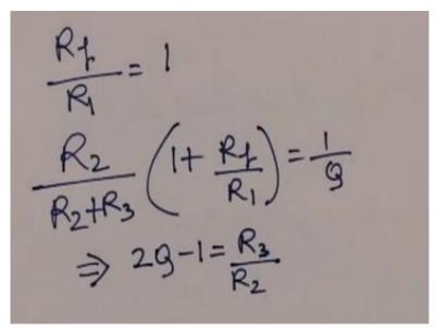
Now of course to equate these 2 equations the values of these R1, R2 and R3 should be such that Rf upon R1 is = 1 R2 upon R2 + R3 1 + Rf upon R1 is = 1 upon Q okay so from here what we get is that the Q value to Q - 1 should be = R3 upon R2 so if we choose our Rf, R1, R2 and R3 according to this equation then we can implement this now once circuit that I did not mention which is frequently used for gain control in an active filter is a what is called a buffer amplifier.
