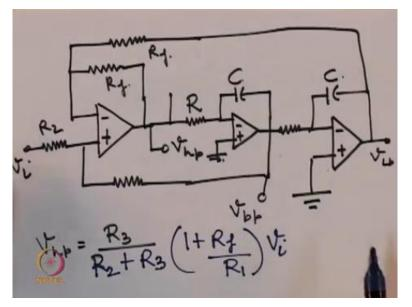
So this circuit is implement this signal flow graph is implemented by the following circuit, so this is my circuit these are the various points at which I obtained by high pass band pass and low pass signals and the output equation that we get if we follow the opamp analysis will be something like this.
