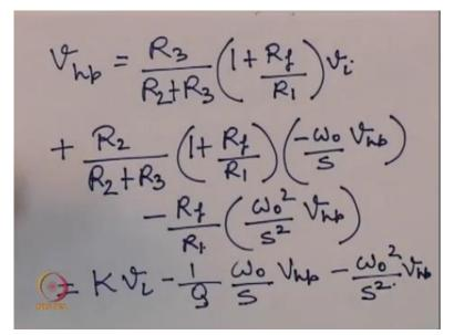
So this V high pass will be = R3 upon R2 + R3 1 + Rf upon R1 Vi + R2 upon 2 + R3 okay, so this is of the same form as Vhp - ok here this gain from the these capacitor based opamps,
