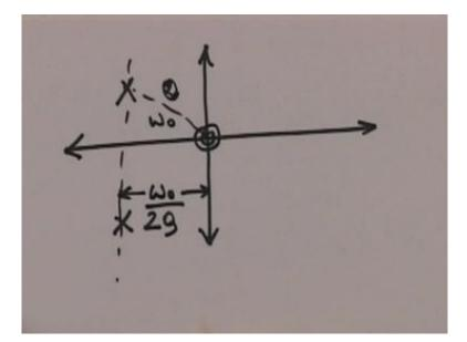
Now the pole positions again are like this two 0's at the origin and the pole locations are the same as for a low pass prototype ok and finally for the band pass prototype, now the reason I am elaborating on these transfer functions is that we will see certain similarities in their transfer functions eventually for the band pass prototype.
