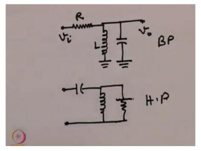
This is a band pass and this is a high pass prototype sorry this is a high pass prototype these 2 circuits can be implemented using this active inductor the low pass cannot be implemented because the low pass prototype has a circuit like this.
