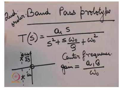
So then for the band pass prototype the pole locations are the same zero at origin and center frequency gain, so for the low pass case we had the gain at zero at DC now for the HF case we had the gain at infinity or high frequency gain and for the band pass filter we have a center frequency gain of this one.
