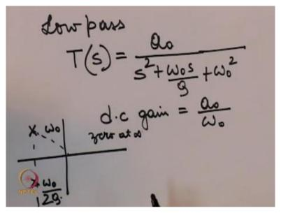
So a low pass second order low pass filter will have a transfer function like this with a dc gain, so the poles are at this position 0 at infinity this radial distance of the pole from the origin is 0 and the horizontal distance from the Y axis for both is like this okay.
