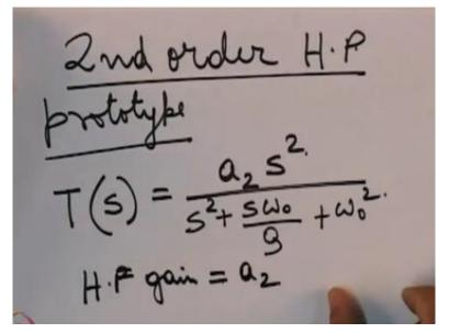
Then for the high pass prototype high frequency or gain at infinity is = A2.
