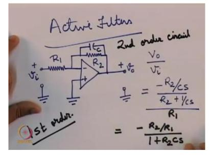
Now one of the simplest implementation of an active filter is using a simple non inverting or inverting open like, so we have so say you have opamp in inverting configuration so here what you see suppose we consider this circuit then you know that Vo upon Vi will be given by - R2 upon Cs by R2 + 1 upon CS this whole upon R1, so this comes out to - R2 upon R1 upon 1 + R2Cs.
