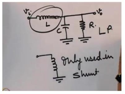
So this low pass prototype has a circuit like this and that active inductor we saw the other terminal always has to be grounded so we have implemented an active inductor but 1 terminal of that inductor is always ground, so it can be used only in shunt it cannot be used in series like we have here and that is the reason we cannot implement a LP or low pass prototype using this inductor of course there are many other implementations of low pass
