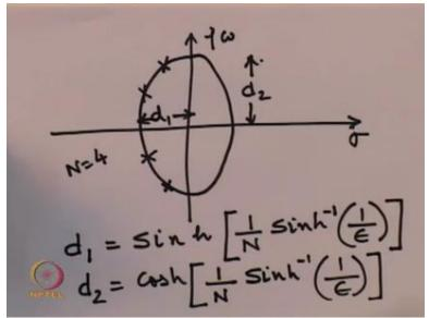
So we can graphically represent the poles like this, this is my complex S plane suppose we have a N = 4 where this say d1 represents the semi minor axis and d2 represents the semi major axis
