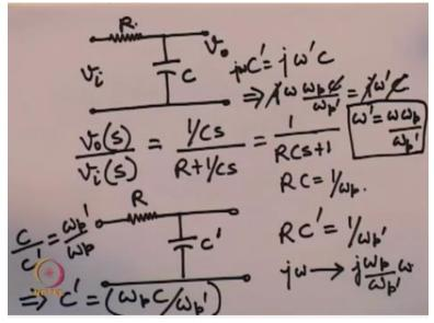
Suppose you have a circuit initially like this okay so here in this case Vo upon Vi in the Laplace domain will come out to and this in turn comes out to 1 upon so here this RC is the 3 db or cutoff frequency is RC is equal to 1 upon omega p where omega p is the 3 db or cutoff frequency.
