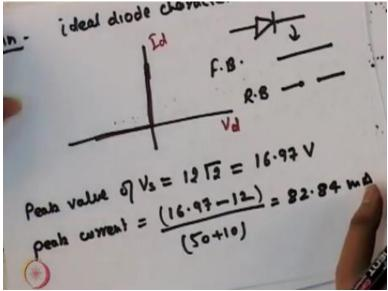
Now going to A part, so A part is asking sketch the diode current wave form for VB = 12 volt. so first let's see and there is one thing given in this circuit assume ideal diodes rather ideal diode, so what is ideal diode characteristics which is like this, so this is sVd this is Id so this is the line graph which means if this is diode in forward bias condition this will be this will be at as short circuit and reverse bias condition this will act as op amp.
