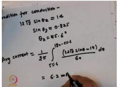
When condition for conduction 12 root 2 Sin theta 2 = 14 Sin theta 2 = 0.825 theta 2 = 55.6 degrees so the average current = 1 upon 2 Phi 55.6 to 180 - 55.6 12 root 2 Sin theta - 14 upon 60 d theta = 6.2 milliamperes this was our problem.
