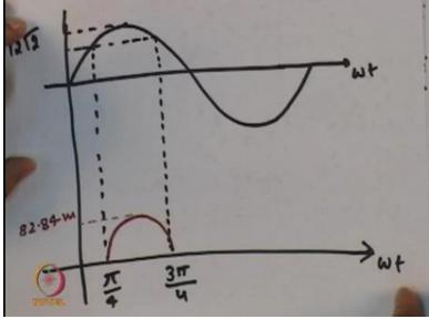
Peak value is 12 root 2 and I am drawing current wave form, so you are having this because this the diode start conducting after Phi by 4 this is the omega t omega t, so the current wave form would be this, this value would be the peak value and all other areas diode will be reverse biased conducting so this is the wave form of current now what is the average value?
