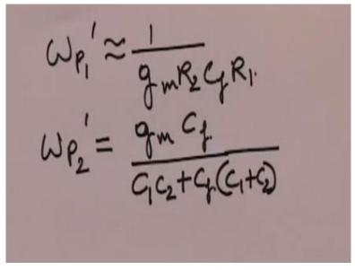
This is 1 pole and this omega p1 can be approximately given as and the other pole is given as, (**Refer Slide time: 17:08**)
