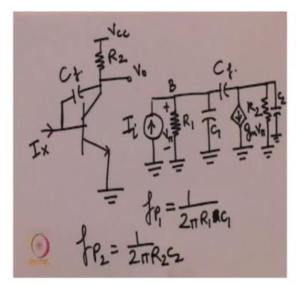
So first of all let us consider a BJT with a feedback capacitor connected between the base and collector, so for now we have not gone into the details of BJT but just understand that it is a 3 terminal device as supposed to a 2 terminal device like a resistance or capacitance or inductance without going into the physics of this BJT I will just state the equivalent model of a BJT which is like this.
