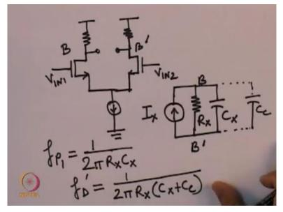
We have something which is known as a differential amplifier which is of this form so this is the supply this is the ground these are the inputs and the outputs are taken from this B B dash now we could write and equivalent small signal model of this circuit like this ok so Rx and Cx are the equivalent shunt resistance and capacitances across the terminals B B dash not that these are the real resistance and capacitance these are just the equivalent.
