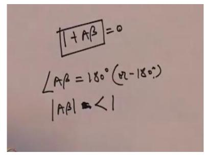
So there are 2 critical features you know, one is that when this angle A beta becomes = 180 degree or -180 degree then we have a potentially unstable case the other issue is that not only should it be 180 degree but the magnitude of A beta should also be less than 1 isn't it only when the magnitude of A beta is less than 1 even if the phase of A beta is = 180 degree the system will continue to be stable on the other hand.
