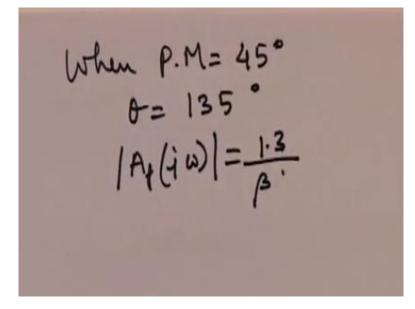
So in that case when theta is = 0 you are closed loop gain magnitude will be = 1 upon 2 beta which is clearly a stable system and when your phase margin is = 45 degree theta is = 135 degree and A of f j omega is = 1.3 over beta which is again a stable system.
