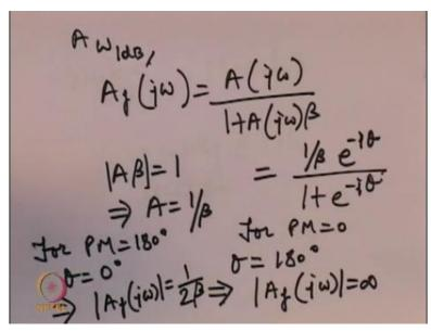
Let us use a sample calculation and see what should be the limit on my magnitude so at omega 1 db ok we have Af of j omega is = A of j omega upon 1+A of j omega beta now A of j omega is A beta = 1 at omega 1 db this implies A is simply = 1 upon beta therefore this equation becomes 1 upon beta e raise to -j theta okay where theta is the value of the phase at omega actually I should have written this way okay.
