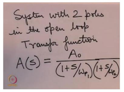
let us now do the same analysis for a system which has more than one poles let us first see a system that has 2 poles in the open loop transfer function, so such a system will have an open loop transfer function like this the characteristic equation will be given like this.
