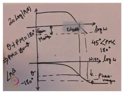
Now while discussing the feedback of a system, recall that we saw that the new denominator I mentioned that the stability of the system is dependent on the characteristic equation 1+A beta = 0.
