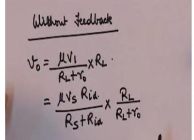
So this is an example of what we call voltage-voltage feedback it is a negative feedback but the type of negative feedback is voltage-voltage ok, so then what do we see what we see here is The output voltage V0 is given by mu V1 upon RL + r0 times RL which in turn is = mu Vs Rid upon
