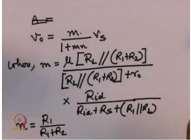
And this N is given as like this, now another effect of feedback which I did not discussed in the previous module was that the output and input impedances depending on of the kind of feedback that is provided the output and input impedances are also modified so for a voltage amplifier as you know.
