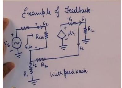
In this module let us see an example of feedback that is applied to a circuit suppose we have a circuit like this now the circuit this is with feedback and the circuit without feedback is like this. (**Refer Slide Time: 02:50**)
